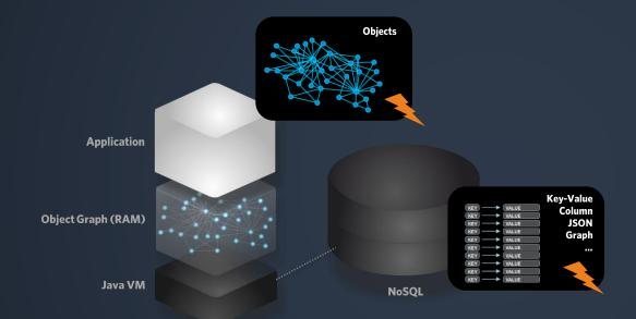
ALL NoSQL data structures are also incompatible with Java object graphs. Even OO and Graph DBs are incompatible with Java object graphs. Impedance Mismatch !
