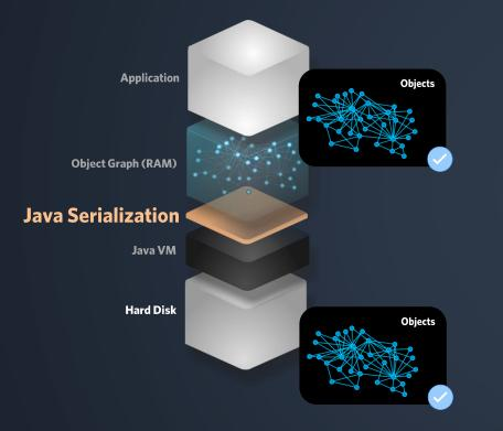
Loading only single objects or subgraphs ondemand and updating the object graph automatically, is not covered by the Java serialization. Additionally, Java serialization is limited and slow. Beyond serialization, there are numerous challenges in terms of persistence that are not covered by Java serialization.
