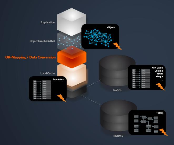
Even though reading data from a local cache, mapping/conversion is required.
